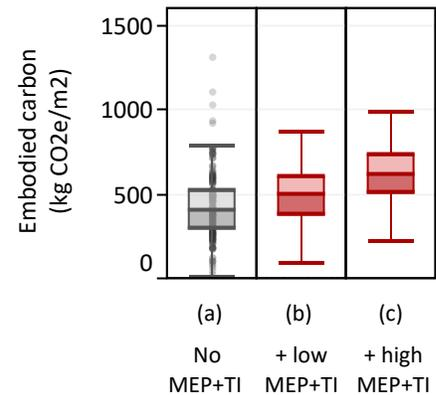
Figure 3. Results from the Embodied Carbon Benchmark Study, filtered for building use type = office buildings; scope = structure, foundation, and enclosure; life cycle stages = A1-A5. Three variations are shown: (a) the original ECB values; (b) original values + low MEP TI estimates; and (c) original values + high MEP TI estimates.
